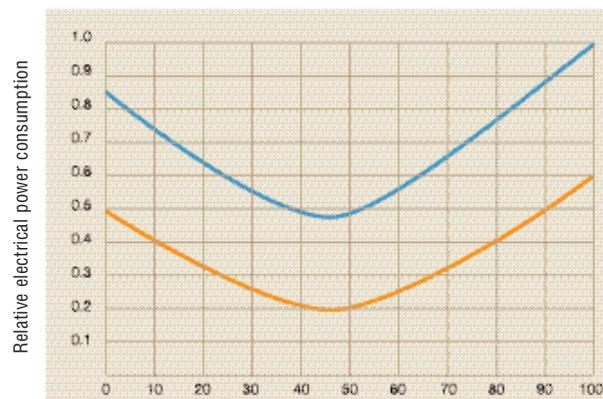
Percentage of car loading. Calculated on the basis of a lift with a load of 630 kg - speed 1.00 m/s with 150 start-ups per hour.
